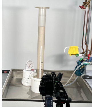
Figure 1: (a) Schematic representation of the setup of two simple one-dimensional tests on an initially dry fine-sand sample. (b) and (c) experimental setup for capillary rise and infiltration, photos: Riemenschneider [65].
