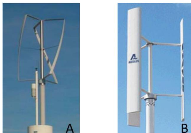
Source: A - Helical VAWT (Turby by Turby b.v. ([www.turby.nl](http://www.turby.nl))). B - H-Darrieus rotor VAWT (Aeolos 1kW by Aelos (<https://www.windturbinestar.com>))
