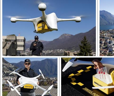
the drone can actually fly as far as 20 km, which means Ticino EOC is already considering a future possibility of transporting laboratory samples from other hospitals even further away.
